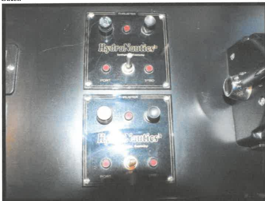
HydraNautics both bow and stern-Not connected at time of survey.
